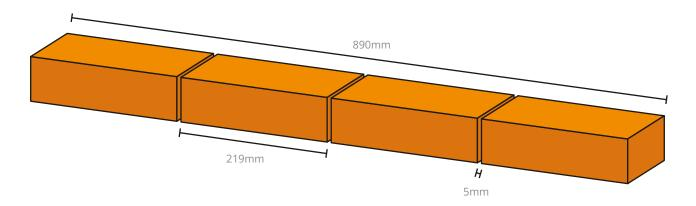
As demonstrated, by maintaining the designated CO of 225mm (by varying the average mortar joint to suit the brick size in construction), ensures that all brickwork designs based on the CO of 225mm can be achieved without the need for cut bricks.
