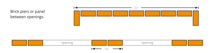
Maintaining module size based on a BSEN771-1 T2 Brick
