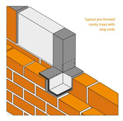
Projects must be evaluated in accordance with exposure requirements this may require increased concentration on workmanship higher mortar strengths and emphasising cappings, coping, DPCs etc.
